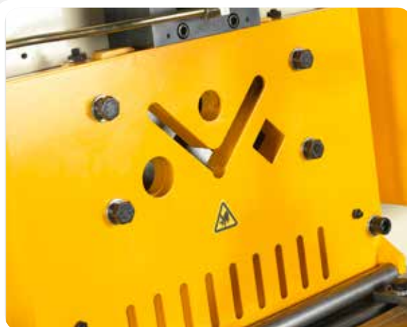
Angle shearing without loss of material. Wide range of openings for Ø, ▢ and L Ø ▢ and ▤ rim cutting station: Stations equipped with an assembly that acts as a hydraulic stop
